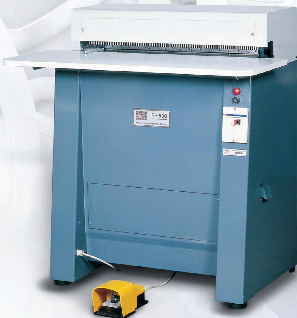
Electric punching machine 800 mm. width
